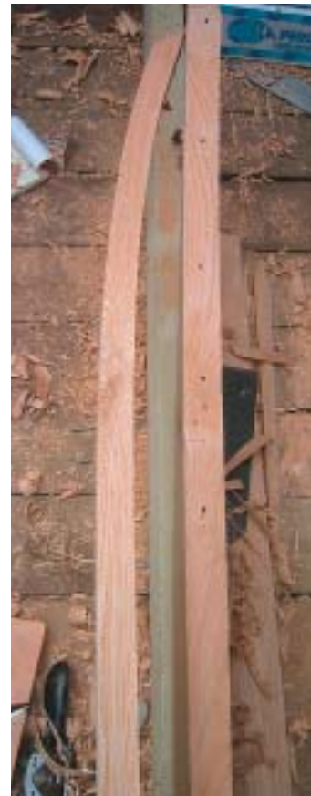
Left & below: Stem and sternposts were cut from large crooks of sweet chestnut, which is stable, light and easy to carve though not very strong. Right: The dovetail-sectioned straight keel is oak.
