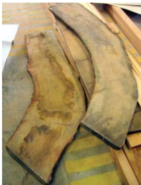
Left & below: Stem and sternposts were cut from large crooks of sweet chestnut, which is stable, light and easy to carve though not very strong. Right: The dovetail-sectioned straight keel is oak.
