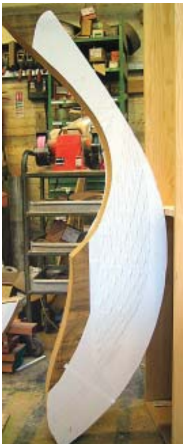
Left & below: Stem and sternposts were cut from large crooks of sweet chestnut, which is stable, light and easy to carve though not very strong. Right: The dovetail-sectioned straight keel is oak.
