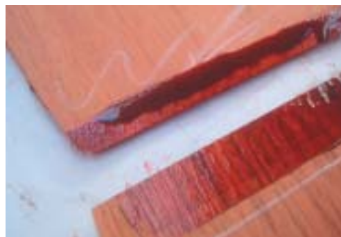
A trial assembly after coating just one of the joint faces with glue confirms good contact.
