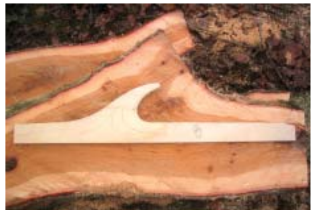
Above: Each plank overlaps the next by 3/4" (20mm). Below: Trying out the pattern for the grown cleat or keber on the first of the oak crooks from Mydhurst. Bottom: The first finished frame cleat.
