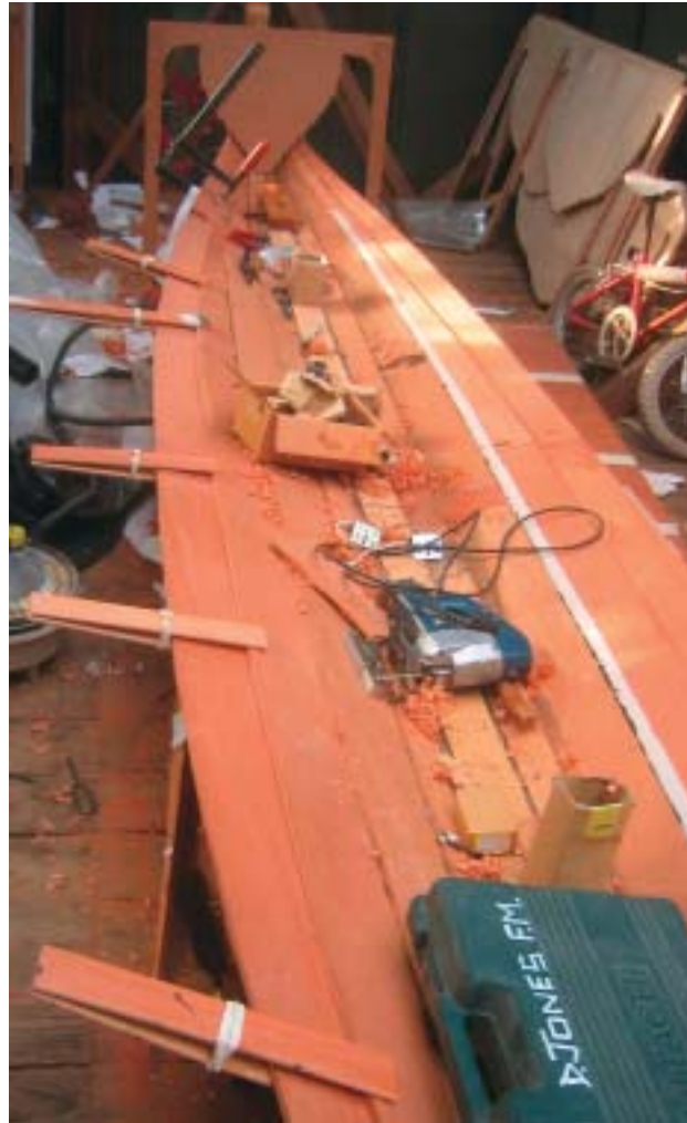
Above: To maintain an adequate curing temperature, the resorcinol glued joint gets its own hot water bottle. Right: Home-made clamps fabricated from bedding slats have enough reach to hold the plank lands together.
