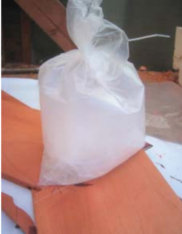
Above: To maintain an adequate curing temperature, the resorcinol glued joint gets its own hot water bottle. Right: Home-made clamps fabricated from bedding slats have enough reach to hold the plank lands together.
